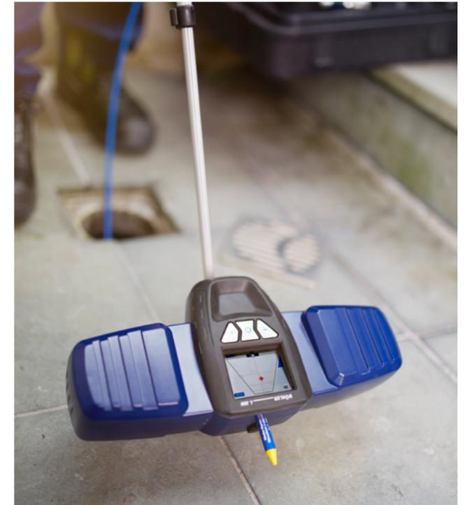
The Wohler L 200 Locator makes it possible to locate the camera head wirelessly.
