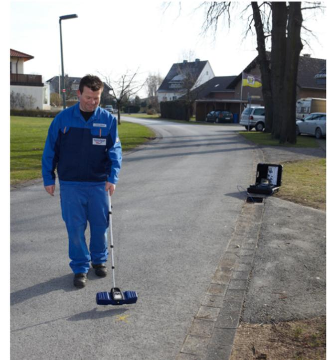
The Wohler VIS 350 precisely locates radio signals transmitted by the camera head through concrete and asphalt to save time and money in repairs.
